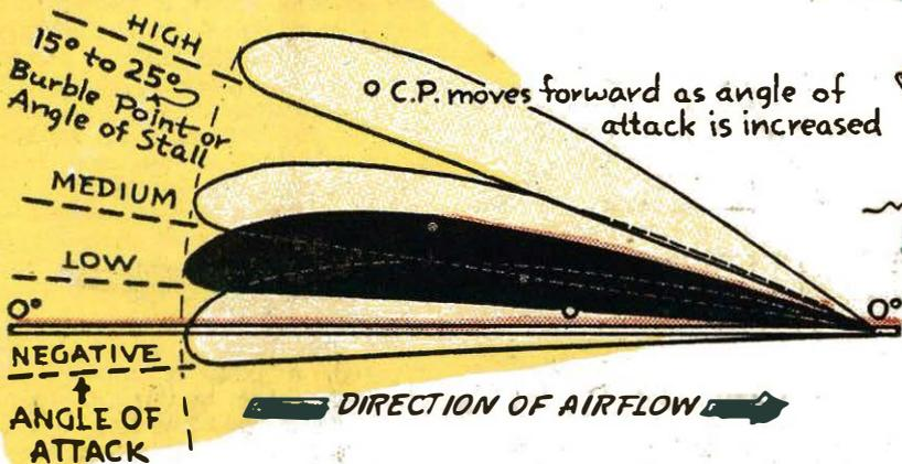
Relative wind operates against the bottom surface of the wing to produce positive air pressure. The direction of the force is upward and backward. That portion of the force which is pushing the wing upward is developing direct air-pressure lift. The portion that is backward in direction is producing wing drag.
