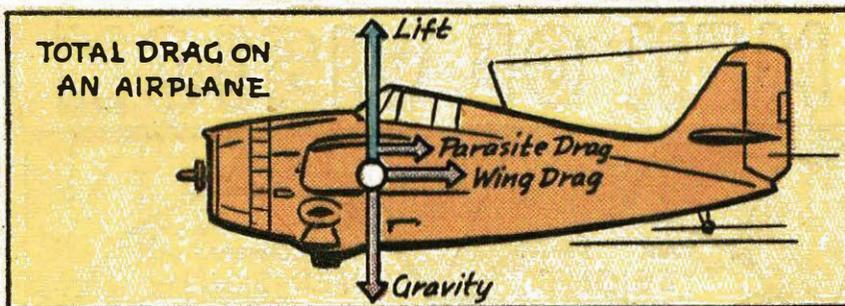
**DRAG RETARDS MOTION** and must be overcome by forward drive or thrust developed by the engine-powered airscrew. Drag created by the lifting surface is called wing drag; that caused by fuselage struts and other parts is called parasite drag. Friction of the wings causes friction drag.
